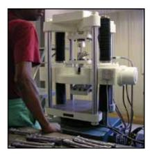
For most users, the standard Super L line includes: 30,000 to 400,000 lbf (150 to 2,000 kN)
