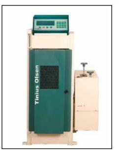
and polished. The upper platen comes with a self-aligning action and suitably sized spacers are also provided as standard to accommodate a variety of different sizes of specimen – the specification table shows which platen set comes with the machine.
