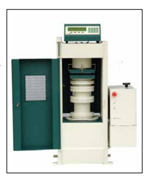
precise control over the load application; a pace rate bar on the display gives operator feedback on the loading rate. The interlocked safety doors on the front and back of the machine prevent the possibility of injury during the test, and a chute is secured to the back of the machine so that once the test is complete, specimen debris can be simply pushed or brushed out. An optional stand is available so these operations can be performed at a safe and comfortable work height.
