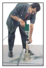
and continues to the inside of diamond core bit. The water jacket surrounding the core barrel is flanged. so it can be clamped to the surface to be drilled with the supplied clamping pliers and anchors. A rubber
