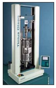
by a PC and software, whereas the S series has a built in display which allows quick simple tests to be performed, in addition to being able to be controlled from a PC and software.
